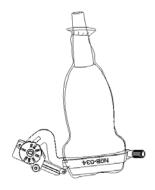
4. Adjust the dial scale to the required needle type shift.
