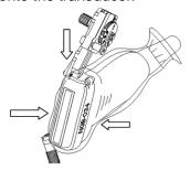
3. Tighten the pinch nut of the needle-guided bracket to confirm that the needle-guided bracket is properly installed on the transducer.
