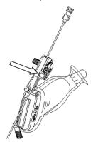
2. Turn over the V-shaped cover to expose the needle. Remove the probe and bracket.
