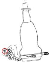
5. Adjust the needle angle to the proper shift as required (loosen the nut first, and then tighten the nut based on the shift you need).
