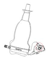
6. Pull the lock pin and close the V-shaped cover to fix the lock pin in the groove of the needle type adjusting base, so as to install the needle into the guiding hole.
