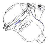
(3) Tighten the pinch nut of the needle-guided bracket to confirm that the needle-guided bracket is properly installed on the probe. Loosen the angle adjusting nut.
