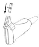
(5) Insert a biopsy needle with the same specification as that of the guiding block into the guiding block hole.
